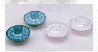
The MGE bacterial filter is a sealed disposable air filter capsule moulded in high impact polystyrene and encapsulates a bonded micro glass fibre disc. The 0.3 micron particle retention of the filter medium gives not less than 99.985% D.O.P. and provides an effective barrier against aerosol contamination.
