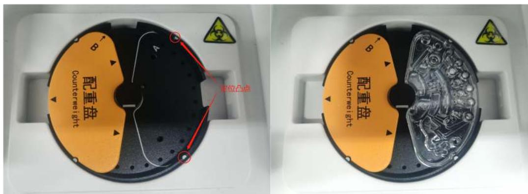
2.4-2 Diagram of reagent disk installation
